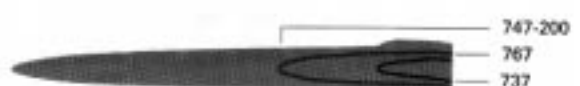
The diagram above indicates that a 767, 737 and similar aircraft leave a significantly smaller imprint than 747-200 series aircraft
