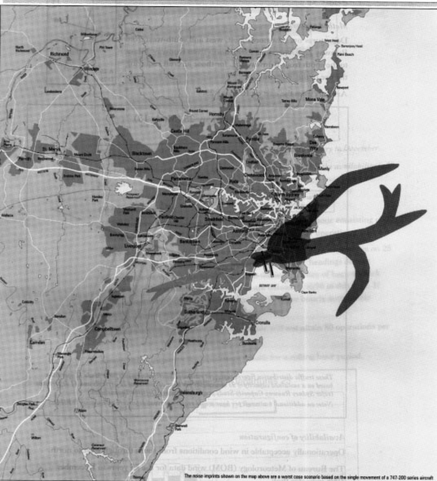
The noise imprints shown on the map above are a worst case scenario based on the single movement of a 747-200 series aircraft
