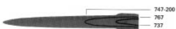
The diagram above indicates that a 767, 737 and similar aircraft leave a significantly smaller imprint than 747-200 series aircraft
