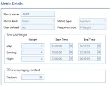
Figure 1: Example setup of ANEF Metric in AEDT
