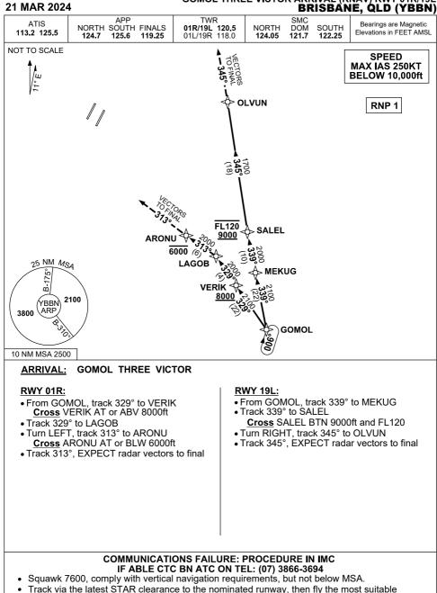
Track via the latest STAR clearance to the nominated runway, then fly the mapproach in accordance with ERSA EMERG Section 1.5.
