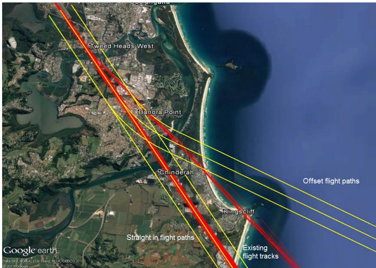
Figure 1: Indicative straight-in and offset flight path corridors for aircraft landing onto runway 32 (yellow) and existing arrival tracks (red) to show the change to the offset flight path
