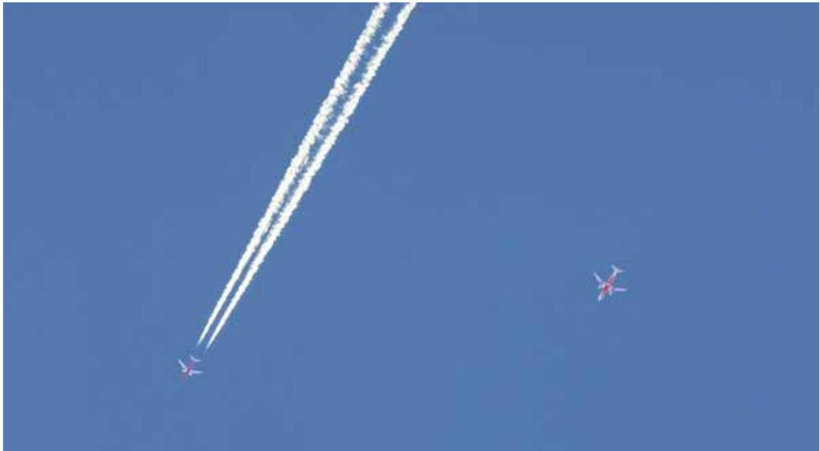
**Above:** Figure depicts two aircraft on the same track, at different altitudes, one creating a condensation trail and the other not. Highlighting that the atmospheric conditions create the condensation trail.
