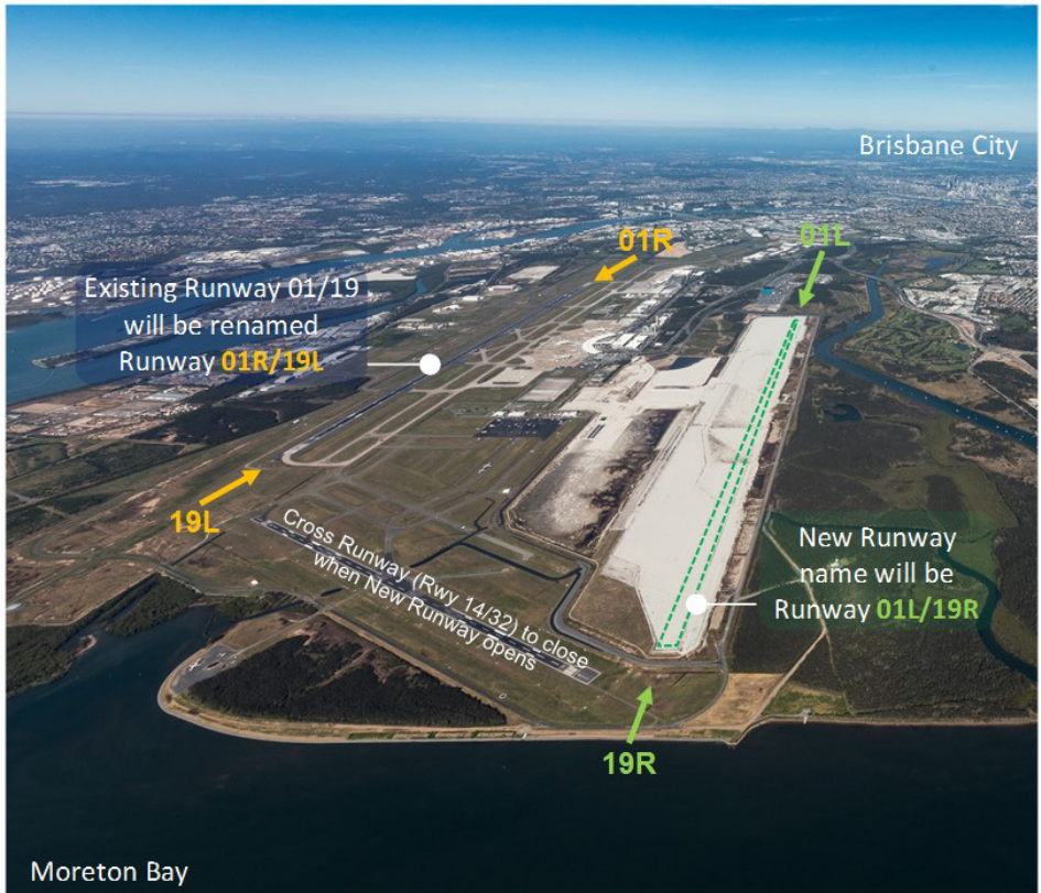
Figure 1: The existing main runway 01/19 will be officially renamed 01R/19L well ahead of the opening of the new parallel runway.
